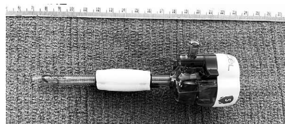
FIG. 2. The novel cleaning device on a 5 mm port.
